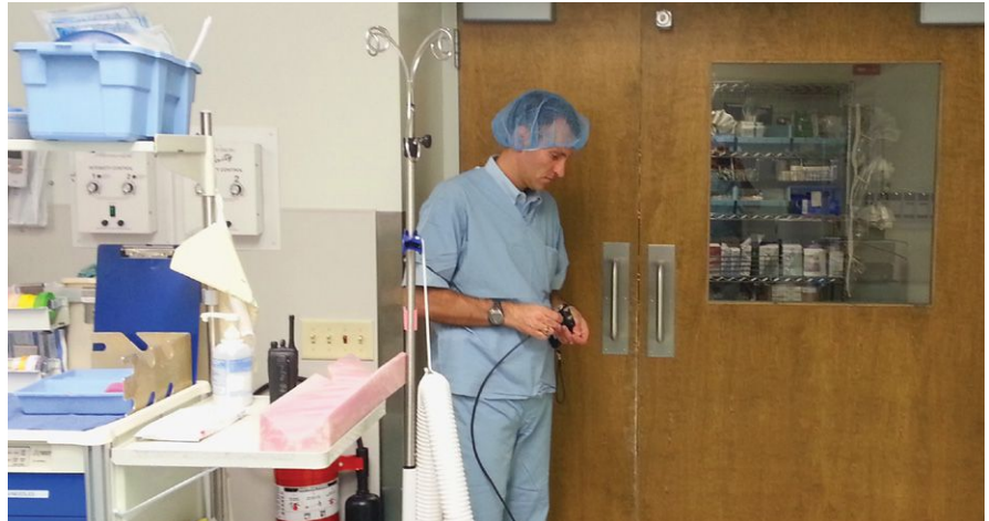
Testing of critical space pressurization is an essential aspect of existing building commissioning in health care facilities.
